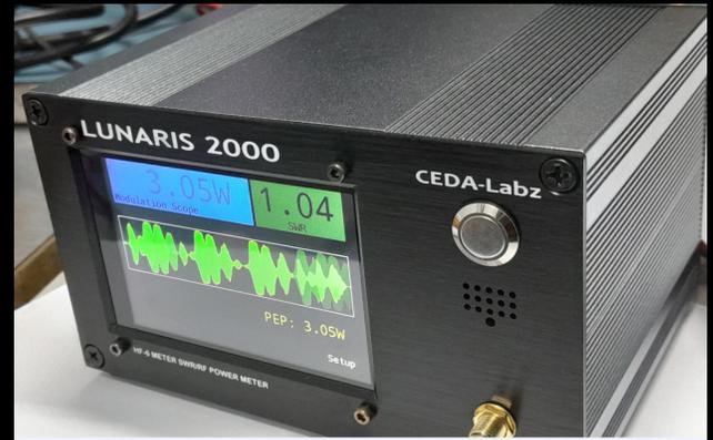
2kW SWR/POWER meter for HF + 6 m Fully auto ranging using ARM CORTEX-M7 & 200 times per second sampling rate. Highly accurate & fast for measuring Forward, Reflected, Peak / Average Power & VSWR. CALIBRATED with ROHDE & SCHWARZ SMY 01 and SMA1008 Signal Generator
