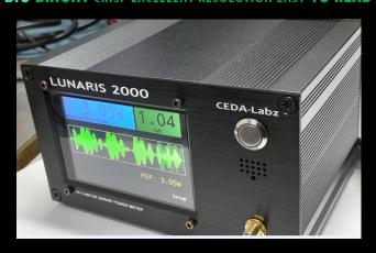
2kW SWR/POWER meter for HF + 6 m Fully auto ranging using ARM CORTEX-M7 &200 times per second sampling rate. Highly accurate & fast for measuring Forward, Reflected, Peak / Average Power & VSWR. CALIBRATED with ROHDE & SCHWARZ SMY 01 and SMA1008 Signal Generator
