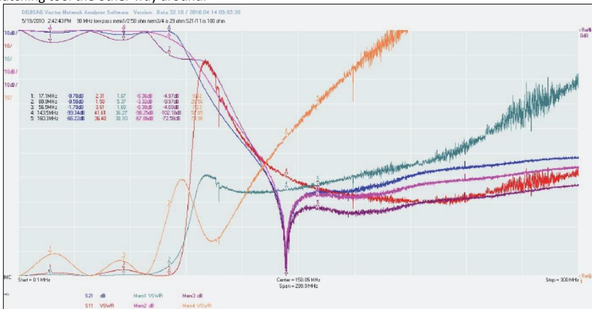
What is important? -A low insertion loss. You do not want the band-pass signals to be attenuated. You also want a steep roll-off so you reach the maximum attenuation as quick as possible. And you want a low VSWR in the band-pass section. Each section you add (so you make a filter with a higher order) adds some extra steepness. This is expressed in dB/octave.
