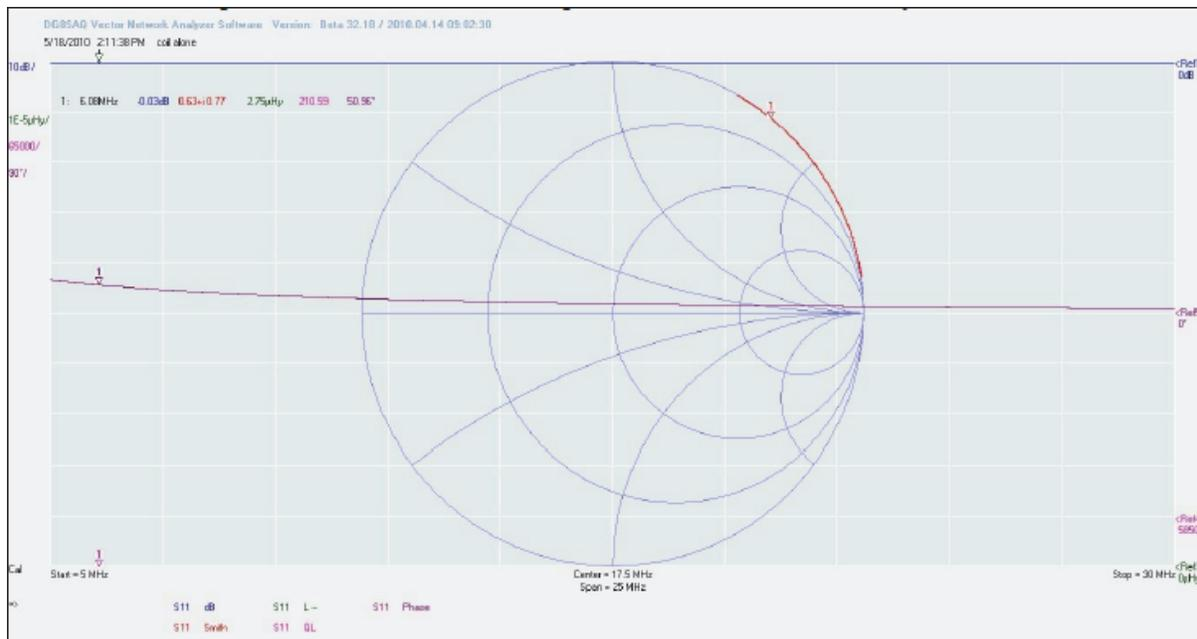
We see here that we have a coil that is 2.75uH. The Q is 210. This is telling us something about the quality of the coil. This tells us the coil has a small real part and so there are not many losses. If the Q was infinite high the energy stored in its magnetic field would stay there forever. It will not dissipate any power. However in the real world there is resistance and loss so the Q will be lower.
