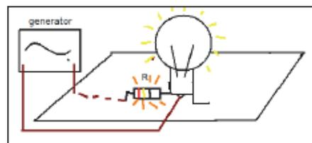
The only problem is the ground. This is not always a perfect conductor. If we go back to our lamp we could see the earth path as having a resistor. The lamp will radiate but not as bright. We lose energy in the resistance of the ground. Practically, this resistance can be really big compared to the total resistance of your system.
