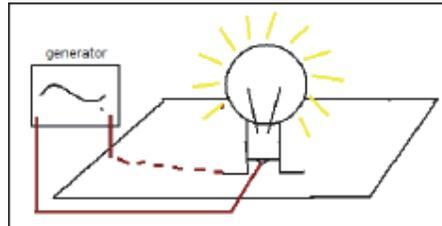
If you use an AC signal this will follow the same route as a DC signal. Now change the light bulb by a capacitor and use a piece of coax from your ac signal source to the lamp. The centre conductor to the capacitor, the braiding to the ground.
