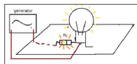
The only problem is the ground. This is not always a perfect conductor. If we go back to our lamp we could see the earth path as having a resistor. The lamp will radiate but not as bright. We lose energy in the resistance of the ground. Practically, this resistance can be really big compared to the total resistance of your system.
